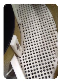
The separation strainer can be made of polyethylene or wire grid. Depending on the type of separation type of machines, the separation sieve is maintained in place with wedges or clamping screws enabling the sieve to be replaced without problems when/if required.
