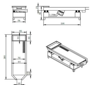
Vibratory separator table Vibra-Sep 1100 L490 For Turbo-Line 120B
