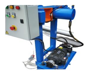
A hydraulic filter press is a piece of equipment used to extract solids from the waste water/compound. The filter press separates the liquids and solids using the pressure filtration where the sewage water/liquid is pumped into the filter press and is dewatered under pressure. Thus, only the solids is being held back in the filter press and the clean compound can be reused.
