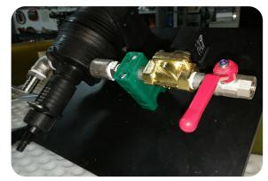
Dosing pump with solenoid and ball valve
