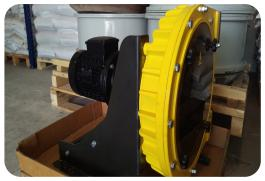
The peristaltic pump which Pers Group recommend is running with an average of 42 rpm @ 50 Hz and pumps 200 L./h. The pump is a 0,55 kW and requires 3 x 400 V AC. The protection class is IP55. The peristaltic pump has the following measurements: L x W x H:  $700 \times 600 \times 500$  mm. and is supplied on 4 pieces of stainless-steel machine feet.
