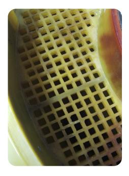
Standard discharge screen made of PU with square holes 20 x 20 mm., can be adjusted with jigsaw to items and media as required. Other size sieves can be required but will then be offered as an optional part.
