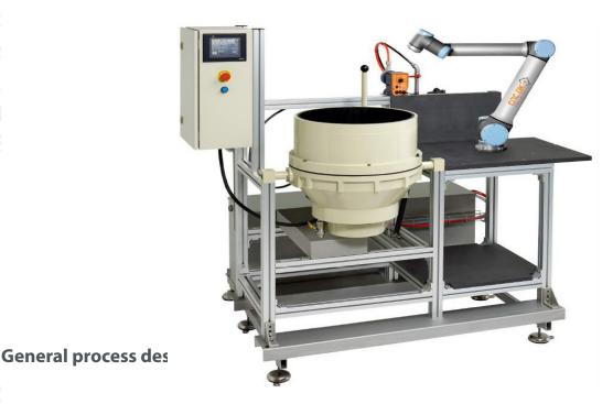
The process is carried out in an open drum/bowl, where the bottom runs around and the ring (side wall) itself is static. In the middle of the gap between the bottom disc and the ceramic ring (both made of hard PU), a ceramic ring is mounted on the casing itself, means that the gap during operation is as low as 0.1 mm. This means that the machine is extremely suitable for polishing e.g. jewellery and very thin items/parts. The machine is delivered with a pre-installed dosing pump.
