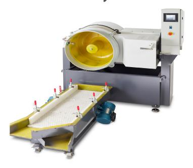
Discharge table Vibra-Sep low model for separating items from media/compound. Under the discharge table there are 2 pcs. of 0.25 kW motors mounted, which provide the actual vibration.
