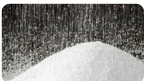
**Glass beads** are a spherical, iron-free blasting medium which is suitable for use with stainless steel and aluminium. The round shape of the product makes it ideal for non-aggressive cleaning and for producing visually attractive surfaces. Micro glass beads are one of the most common reusable blasting media and are used all over the world.
