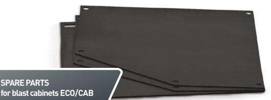
To extend the life of the cabinet enclosure, the interior walls and doors should be lined with rubber curtains. Curtains protect the shell of the blast cabinet from either the direct blast stream and abrasive ricochet. Curtains plates are made of special wear resistant rubber and can be easily installed and replaced when worn.
