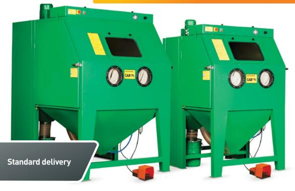
All-welded blast cabinet, ready to use assembled with media recovery hoses, abrasive metering valve, transparent media delivery hose, air hose, GX manual blast gun with GXT-8 tungsten carbide nozzle, lined rubber gloves RGS-800, pilot operated control valve, foot valve with remote control hoses, air filter with manual drain valve, cartridge dust filter, timer operated pulse jet cleaning system, safety and disposable glass window assembly.
